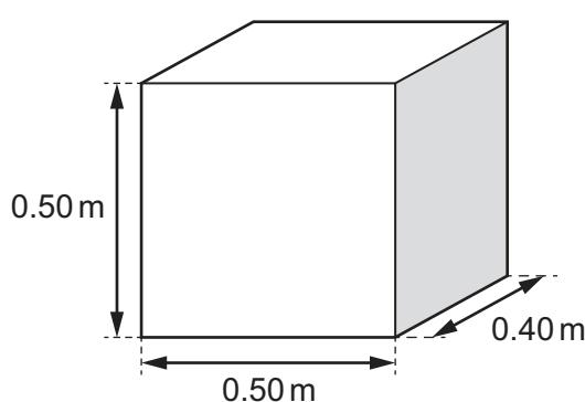
The pressure on the ground due to the weight of the box is 50 Pa.
